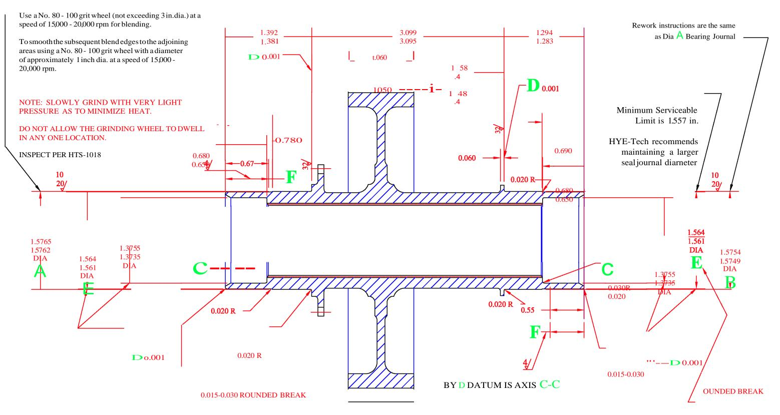
AXIS C-C ESTABLISHED BY DIAMETERS A AND B
